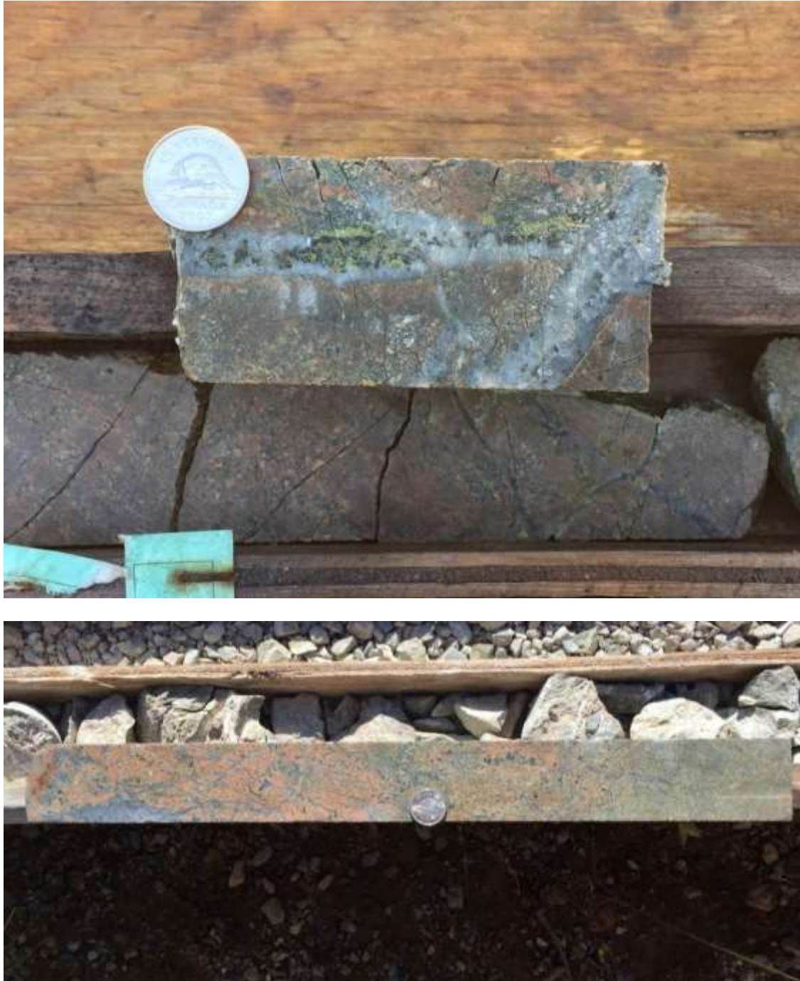
Figure 7-8: Quartz-magnetite-pyrite-epidote veinlets in potassic-altered latite (top: hole BR-03-07@165.95m) and quartz-magnetite±pyrite stockwork in hematite-dusted, weakly potassic-altered to phyllic-altered latite (bottom; hole BR-07-04@226.00m)
