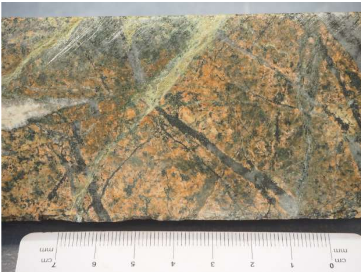
Figure 7-9: Potassic-altered monzonite cut by magnetite-rich granular quartz veinlets, in hole BR-13-01@725.0m.
