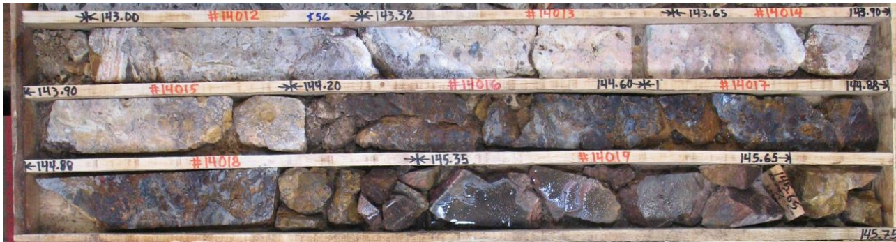
ES-17-16: 143.00 – 145.35m, TW 1.95m 628 g/t Ag, 0.90% Zn, 1.52% Pb Including: 144.20 – 145.35m TW 0.95m 1,133 g/t Ag, 1.56% Zn, 2.98% Pb
